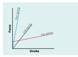
As the piston rod is pressed into the tube, volume reduces and pressure increases. This causes pushing force to increase. In conventional gas springs, this increase is normally around 30% at full compression.
